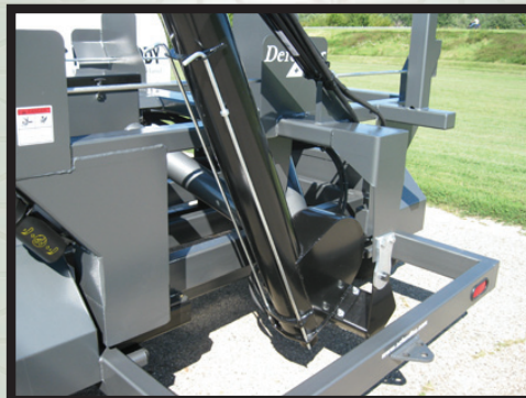
Reversible Auger With Easy Cleanout At Auger Base
